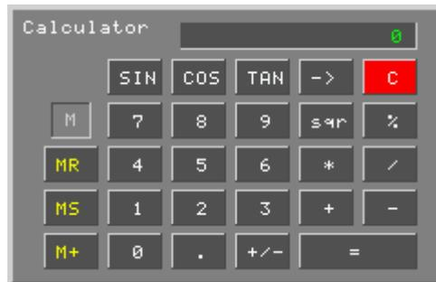
The calculating system is used as a traditional calculator (possible operations are: addition, subtraction, multiplication, division, percentage, square root, sine, cosine and tangent). In addition, the calculator is provided with three memory function keys MS, MR and M+ to temporarily store the result during calculations.
