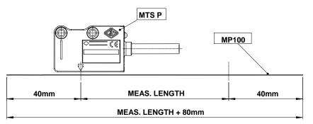
IMPORTANT: in order not to compromise the accuracy of the system, the magnetic band MP100 must be longer than the machine run of at least 40 mm from each side.
